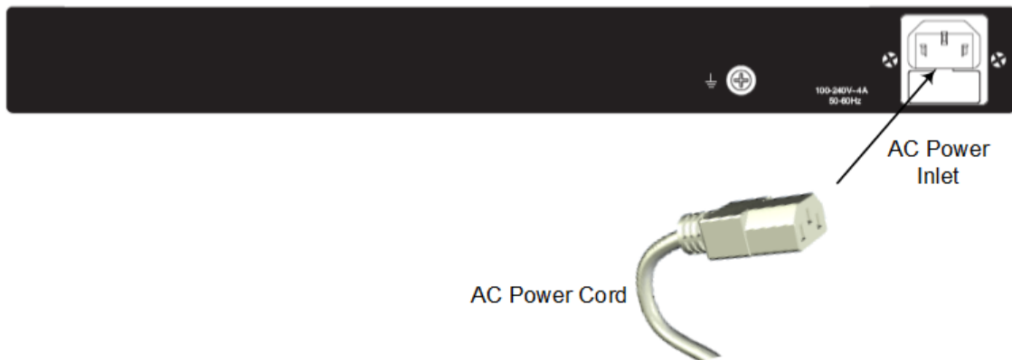
Figure 5-18: Connecting to the Power Supply
