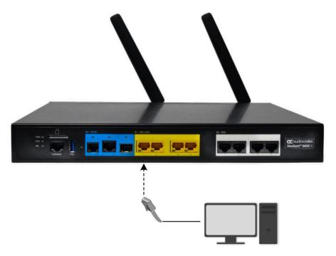
2. Make sure that your computer is configured to automatically obtain an IP address. The device has an embedded DHCP server, which by default, allocates IP addresses to connected computers.
