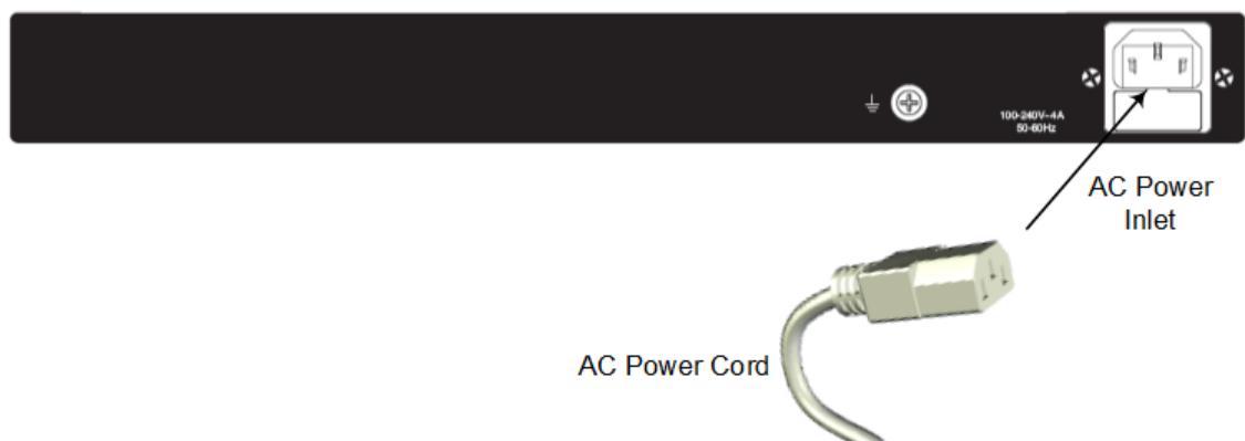
Figure 5-18: Connecting to the Power Supply
