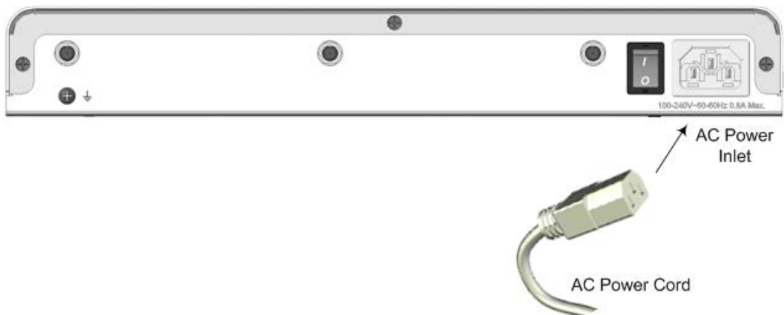
Figure 5-8: Connecting to the Power Supply
