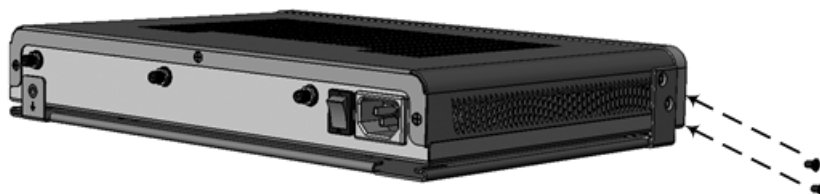
Figure 4-12: Attaching Bracket to Device using Side-Panel Screws
