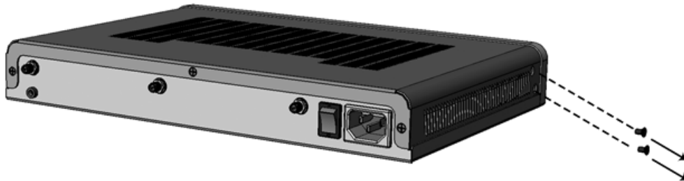
Figure 4-7: Removing Side-Panel Screws
