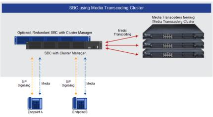
The main benefit of the Media Transcoding Cluster feature is scalability. The Media Transcoder doesn't require licensing of its transcoding resources and allows utilization of all its DSP resources. However, the maximum possible transcoding capacity by the SBC device is according to the License Key of the SBC device, regardless of the number of deployed Media Transcoders.
