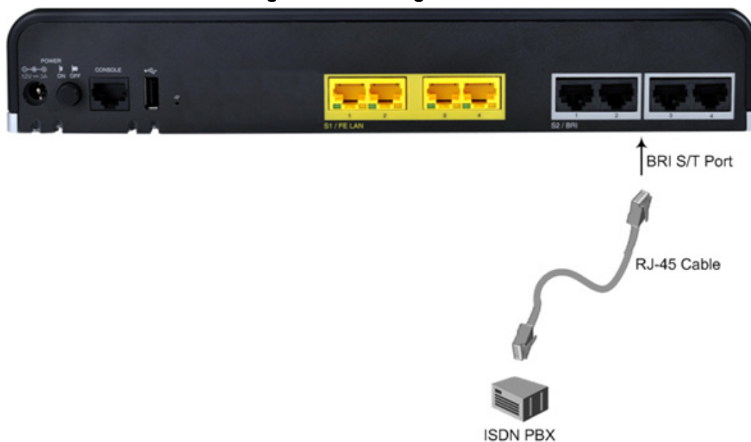
Figure A-1: Cabling BRI Ports
