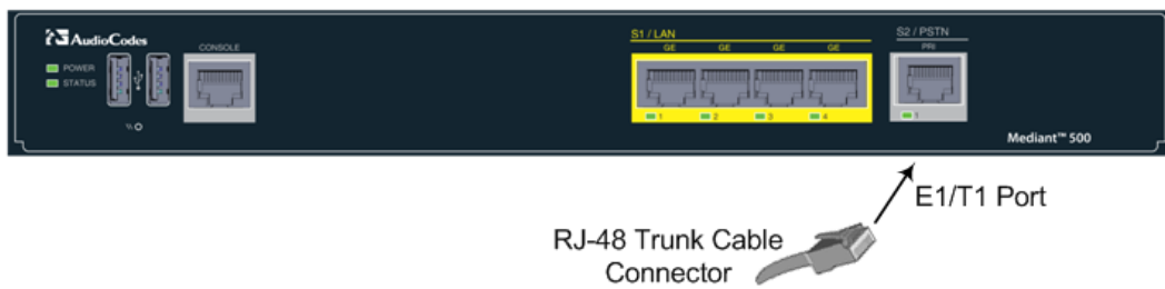
Figure A-2: Mediant 500 Cabling E1/T1 Port
