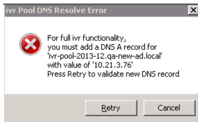
Figure 4-10: ivr pool DNS Resolve Error
