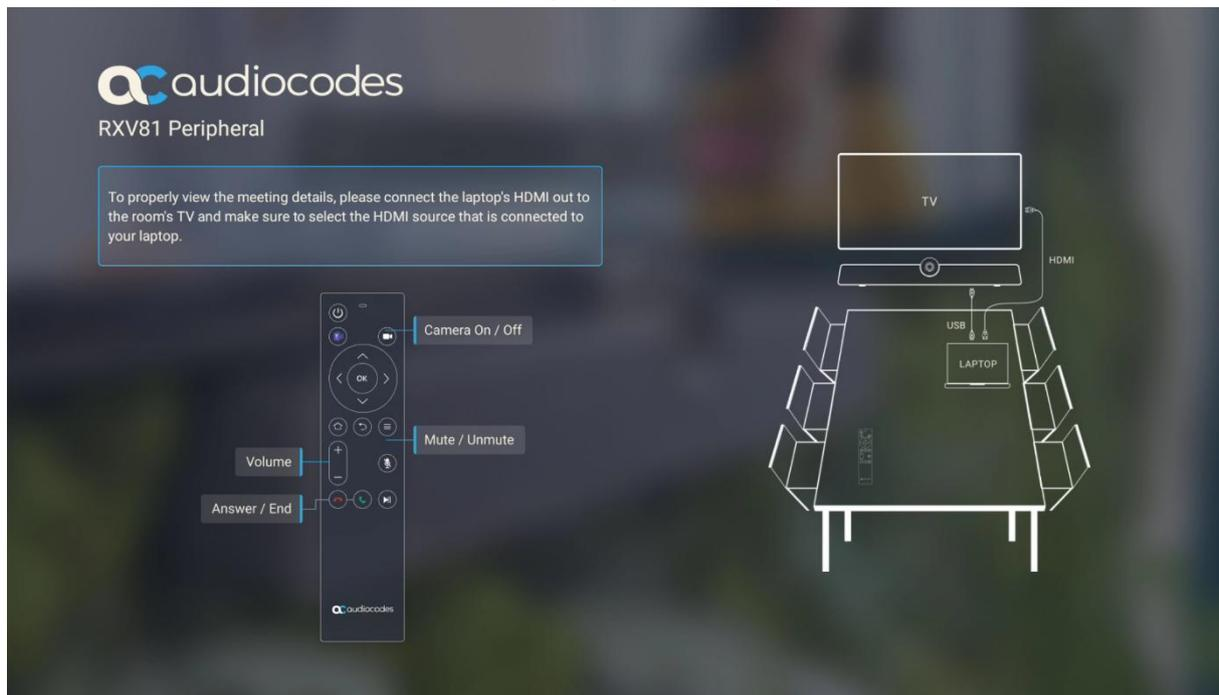
Ad hoc peripheral mode is a versatile feature designed to enhance RXV81 functionality. The mode enables seamless integration of RXV81 with a PC/laptop by utilizing RXV81's audio and camera capabilities as primary audio and camera sources for the PC/laptop.
