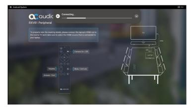
4. Wait until the RC + RXV81 connection is established successfully.
